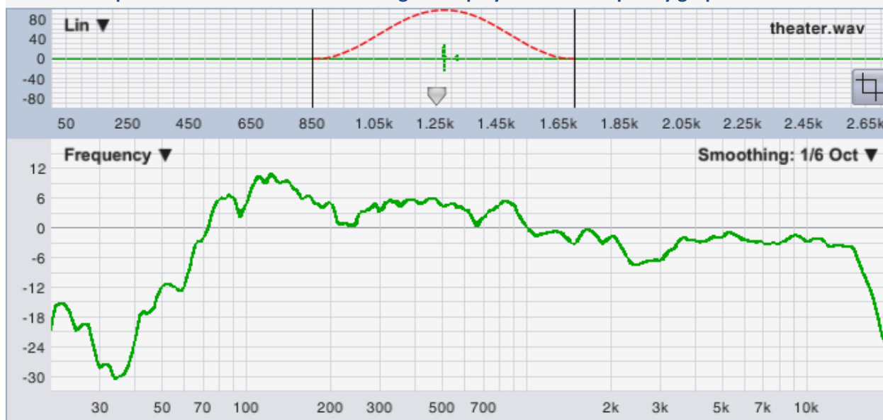
Figure 95: Moving the time 0 point and selecting a time range for display. The time range selected in the navigation pane applies to the Frequency graph as well as time domain graphs (Lin, Log or ETC). Note that Smart uses a tapered data window when transforming any subset of the full IR time range. We've drawn the outline of a Hann window in red on the navigation pane of the "result" portion of the illustration above to help visualize this.
